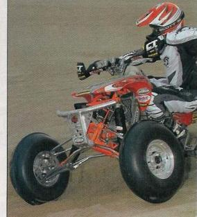
electric start, liquid-cooled, sixspeed, originally designed for a KTM enduro dirt bike. With a 97mm bore, Wiseco 12.5:1 piston, and 6mm Factory KTM stroker kit, the four-stroke leaps up to 576cc. Stronger, freer breathing is accomplished with a 41mm Keihin, Hot Cams and CT stainless exhaust.
